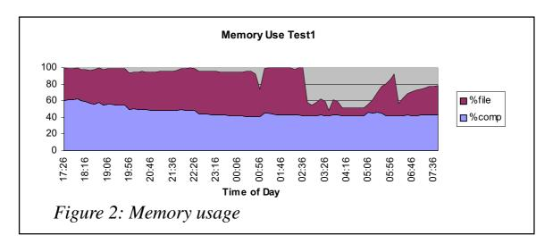
Figure 2 shows a distribution of usage of memory between file and computational (executable program ) pages.
