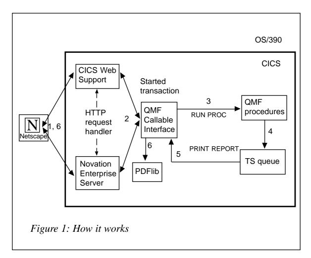
requested, calls the PDFLIB routines to build it (6), builds the HTTP header (see below), and puts the result in the DFHCOMMAREA. The HTTP request handler sends it back to the user (7).
