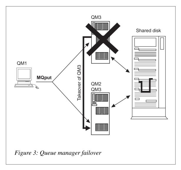
restart and runs a script or program on a standby processor to restart the queue manager there. On the standby processor, the queue manager reads the transaction log and recovers to the point where the failure occurred.
