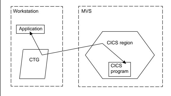
Figure 1: Idealized CTG and CICS workststation configuration
