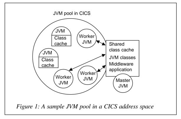
Figure 1 demonstrates a sample JVM pool in a CICS address space. CICS supports one active shared class cache in each region. Use of the shared class cache improves the performance of JVMs in two respects:
