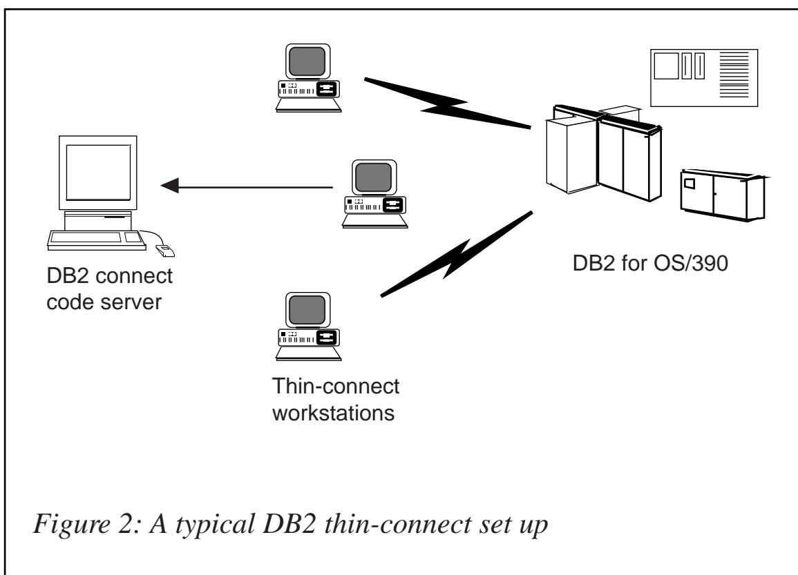
Figure 2: A typical DB2 thin-connect set up
